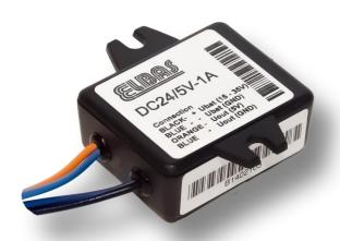
The modern HI DC-DC DC pulse converter with high efficiency up to 95% is designed to power consumers with power supply 5V max 1A. The advantage of this converter is a very small heat loss radiated to the surroundings. The inverter is connected to the 24V on-board network and is protected against short-circuit over voltage in the on-board network. The drive provides 5W output power.
